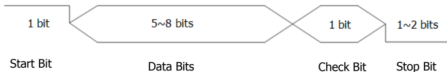
Figure 5-13 Schematic Diagram of RS232 Protocol
